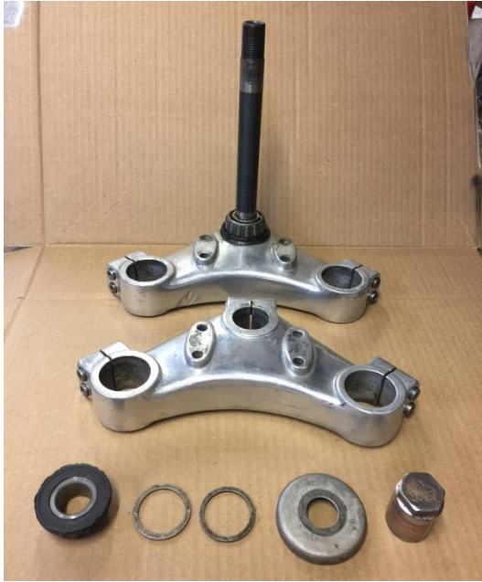
The fork stop on the BSA frame will need to be removed and "stop bars" added to the forks
