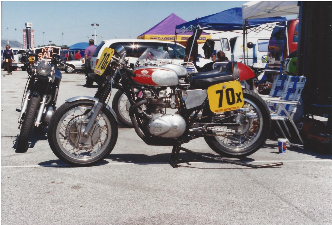
Later machine with two into pipes (from a Boyer design) and special oil tank (oil in frame not used)
